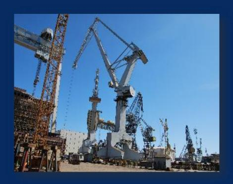
**KONE Cranes** Lifting capacity: Each of 150 tons
