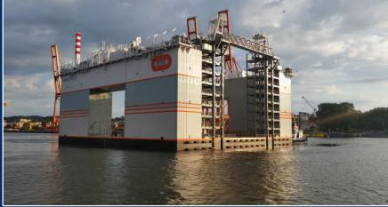
The Floating Dock is specially designed for the construction of concrete caissons and is designated to build a new shore lane in Monaco.
