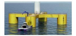
**NAUTILUS Floating Solutions** has developed a floating foundation for offshore wind energy that presents an optimized semisubmersible four-leg design, that will allow the reduction of the LCOE from current designs.
